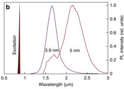
**Fig. 2 IR-emitting HgTe QDs. a** TEM images of the HgTe QDs used in this study (scale bar is 20 nm); insets show a magnified view of selected QDs (scale bars are 5 nm). **b** Emission spectra of HgTe QDs with average sizes of 3.9 and 5.0 nm. Also shown is the spectral position of the PL excitation at 880 nm
