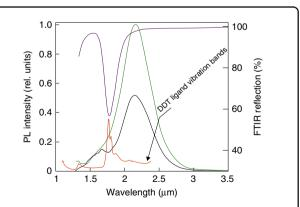
**Fig. 4 Tailoring the IR emission spectra of the HgTe QD film with a laser-printed plasmonic array.** Emission spectrum of the 5.0-nm size HgTe QD layer deposited on a reference Si substrate (black) and a plasmonic nanobump array (green). Also shown are a normalized FTIR reflection spectrum of the corresponding plasmonic nanobump arrays coated with the QD layer (purple) as well as part of the near-IR absorption spectrum of the DDT ligand of the HgTe QDs (red)
