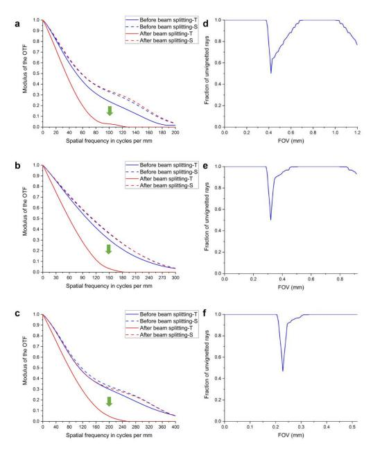
Supplementary Figure S3 Reduction in resolution and illumination due to spectroscopic effects. a–c Simulated resolution reduction at the field-of-view (FOV) intersection of centre and edge channels at magnifications of  $9\times$ ,  $13\times$ , and  $18\times$ . d–f Simulated fraction of unvignetted rays at different FOVs (or object heights) with magnifications of  $9\times$ ,  $13\times$ , and  $18\times$ .
