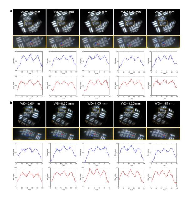
**Supplementary Figure S9 Resolution test with different working distances (WDs) at initial magnification of 13×. a** Resolution test results of the centre channel with different WDs at initial magnification of 13×. **b** Resolution test results of the edge channel with different WDs at initial magnification of 13×.
