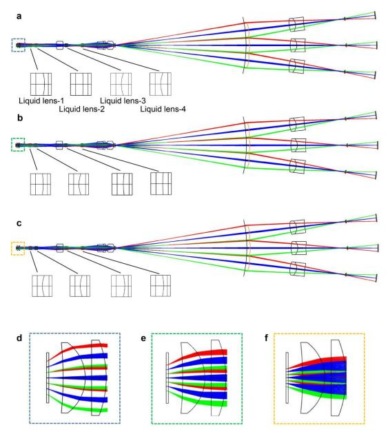
Supplementary Figure S1 Optical path simulation of the proposed microscope. a–c Simulated optical path of the microscope at magnifications of  $9\times$ ,  $13\times$ , and  $18\times$ . d–f Local enlarged images of the simulated optical path at magnifications of  $9\times$ ,  $13\times$ , and  $18\times$ .
