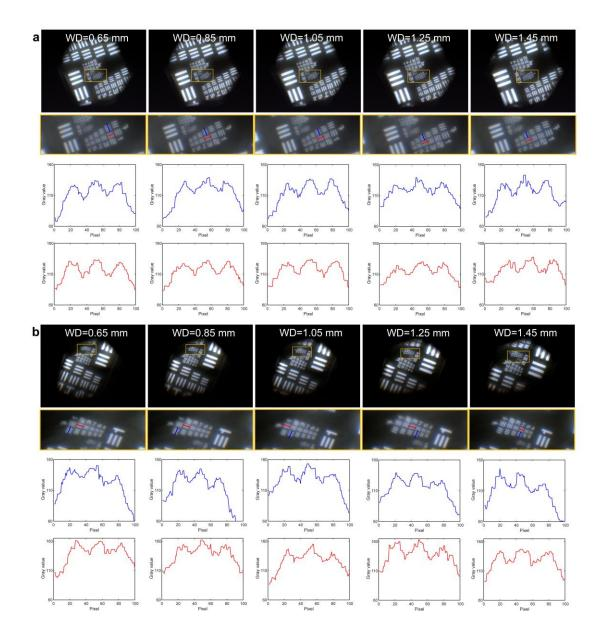
Supplementary Figure S8 Resolution test with different working distances (WDs) at initial magnification of  $9\times$ . a Resolution test results of the centre channel with different WDs at initial magnification of  $9\times$ . b Resolution test results of the edge channel with different WDs at initial magnification of  $9\times$ .
