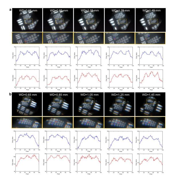
**Supplementary Figure S10 Resolution test with different working distances (WDs) at initial magnification of 18×. a** Resolution test results of the centre channel with different WDs at initial magnification of 18×. **b** Resolution test results of the edge channel with different WDs at initial magnification of 18×.
