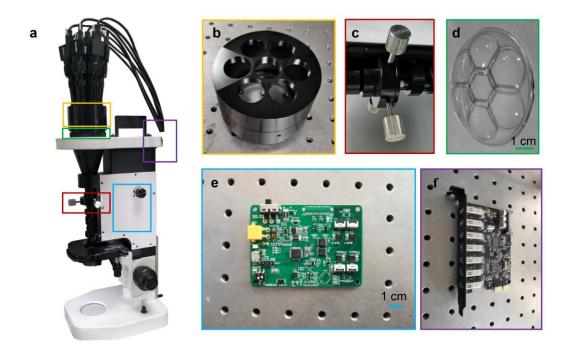
Supplementary Figure S5 Fabrication of the proposed microscope. a Real image of the proposed microscope. b, c Real images of the assembly and adjustment mechanisms. d Real image of the compound eye lens. e Real image of the liquid lens driver. f Real image of the seven-channel data stream transmission port.
