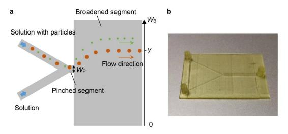
Supplementary Figure S13 Principle and structure of the microfluidic chip for separation of particles. a Principle of the microfluidic chip for separation of particles. b Real image of the microfluidic chip.
