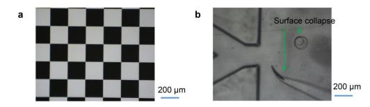
Supplementary Figure S14 FOV of an ordinary microscope. a Chequerboard image captured by the commercial microscope with  $10 \times$  objective lens. b Microfluidic chip image captured by the commercial microscope.
