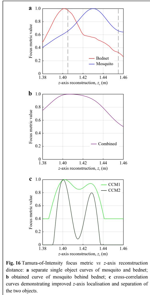
**Fig. 16** Tamura-of-Intensity focus metric vs  $z$ -axis reconstruction distance: **a** separate single object curves of mosquito and bednet; **b** obtained curve of mosquito behind bednet; **c** cross-correlation curves demonstrating improved  $z$ -axis localisation and separation of the two objects.
