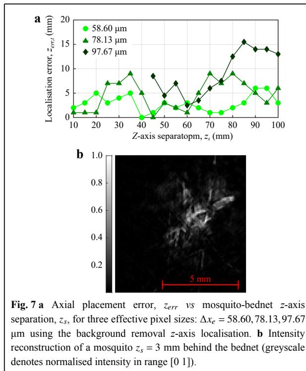
**Fig. 7 a** Axial placement error,  $z_{err}$  vs mosquito-bednet  $z$ -axis separation,  $z_s$ , for three effective pixel sizes:  $\Delta x_e = 58.60, 78.13, 97.67 \mu\text{m}$  using the background removal  $z$ -axis localisation. **b** Intensity reconstruction of a mosquito  $z_s = 3$  mm behind the bednet (greyscale denotes normalised intensity in range [0 1]).
