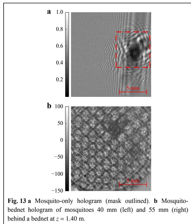
**Fig. 13** **a** Mosquito-only hologram (mask outlined). **b** Mosquito-bednet hologram of mosquitoes 40 mm (left) and 55 mm (right) behind a bednet at  $z = 1.40$  m.
