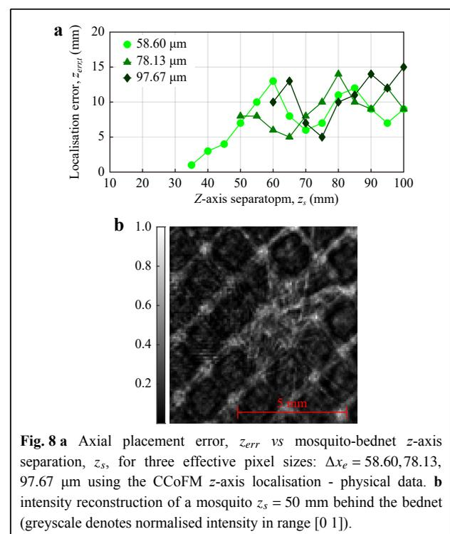
**Fig. 8 a** Axial placement error,  $z_{err}$  vs mosquito-bednet  $z$ -axis separation,  $z_s$ , for three effective pixel sizes:  $\Delta x_e = 58.60, 78.13, 97.67 \mu\text{m}$  using the CCoFM  $z$ -axis localisation - physical data. **b** Intensity reconstruction of a mosquito  $z_s = 50$  mm behind the bednet (greyscale denotes normalised intensity in range [0 1]).
