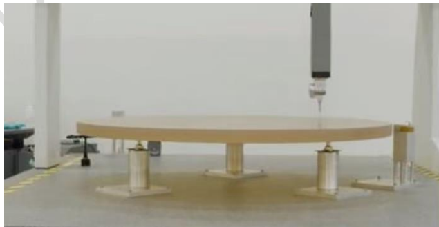
Fig. 32 CMM used in ELT mirror blank measurement. 139
