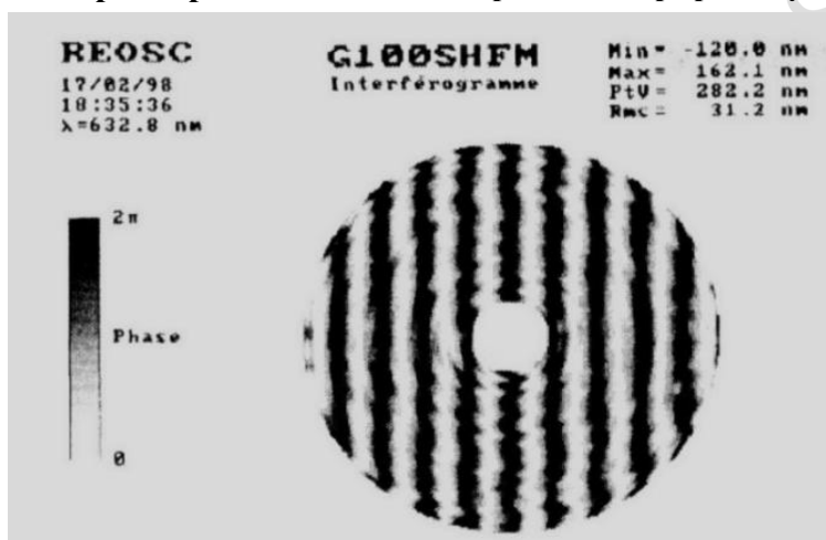
Fig. 54 Interferogram of the Gemini primary mirror testing. 189
