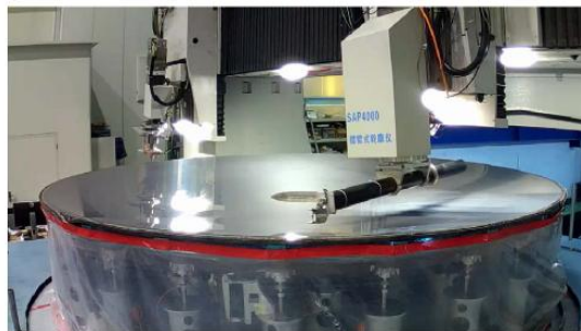
Fig. 36 Surface figure characterization of a 4 m aspheric mirror via swing-arm profilometry (SAP) testing. 21
