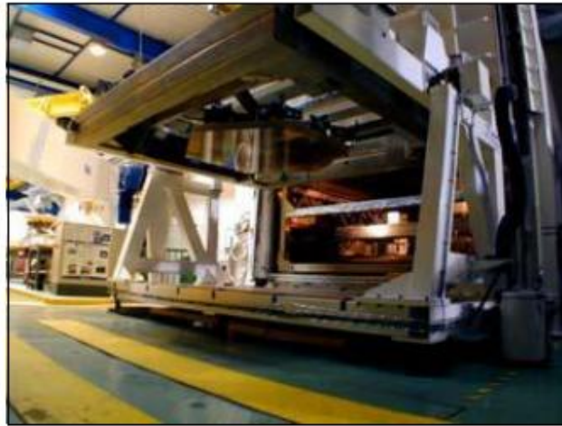
Fig. 20 GTC primary mirror undergoing ion beam shaping. 108
