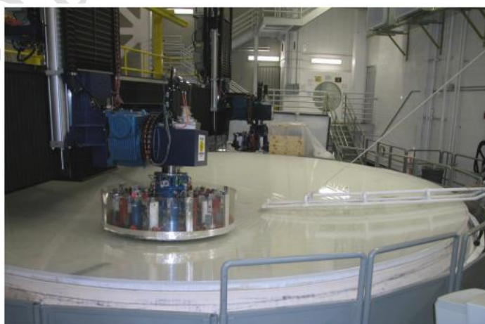
Fig. 12 Stressed-lap polishing of the second LBT mirror on the new 8.4 m polisher. 82
