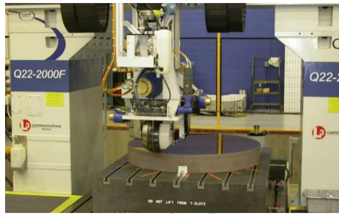
Fig. 14 Q22-2000F MRF polishing machine, commissioned in July 2008, used for 1.5 m diameter optics.
