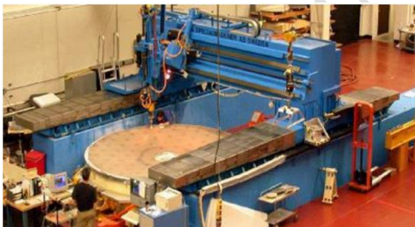
Fig. 11 Primary mirror being optically fabricated using Goodrich's large computer-controlled grinding and polishing machine. 9
