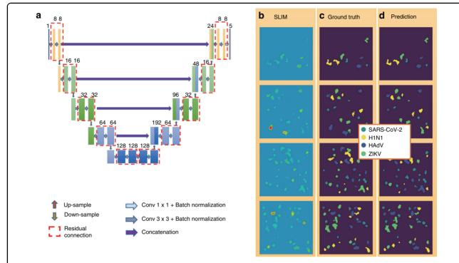
Fig. 5 Training a deep neural network to perform classification of virus particles for the second dataset. **a** We used a modified version of U-Net for this semantic-segmentation task. Besides reducing the number of parameters in the network to around 0.8 million, we also added in residual connection and batch normalization for faster convergence. Model inference on images from the test set. **b** Synthesized images of mixed virus particles. **c** Ground truth label. **d** Model inference
