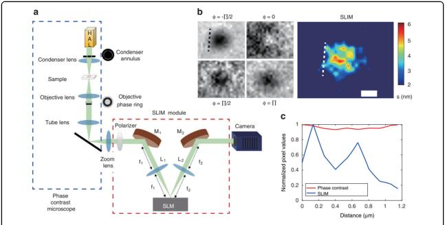
Fig. 2 SLIM. a Optical configuration of SLIM. **b** Image reconstruction, with color bar representing optical path length (s), in nm. **c** Profile through yellow dotted line in **b**, showing high sensitivity of SLIM over phase contrast
