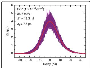
Fig. 4 An example transient output pulse energy ( $E_3$ ) as a function of delay between the input pulses (the  $k_1$  and  $k_2$  beams) for one of the Si:P samples far from resonance. The signal is a third-order autocorrelation of the pulse temporal profile. This autocorrelation signal appears Gaussian to a good approximation (red line) with r.m.s. width  $\sigma_t = 7.5$  ps, so the inferred r.m.s. duration of the pump beams is  $t_0 = \sqrt{2/3}\sigma_t = 6.1$  ps
