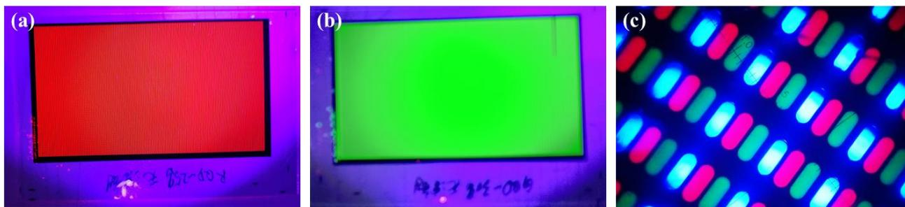
**Fig. S9** Photographs of (a) red and (b) green CdSe patterns under excitation by UV light. (c) Red, green and blue pixel patterns illuminated by blue backlight.
