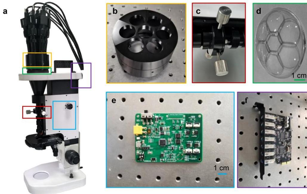
**Supplementary Figure S5 Fabrication of the proposed microscope.** **a** Real image of the proposed microscope. **b, c** Real images of the assembly and adjustment mechanisms. **d** Real image of the compound eye lens. **e** Real image of the liquid lens driver. **f** Real image of the seven-channel data stream transmission port.
