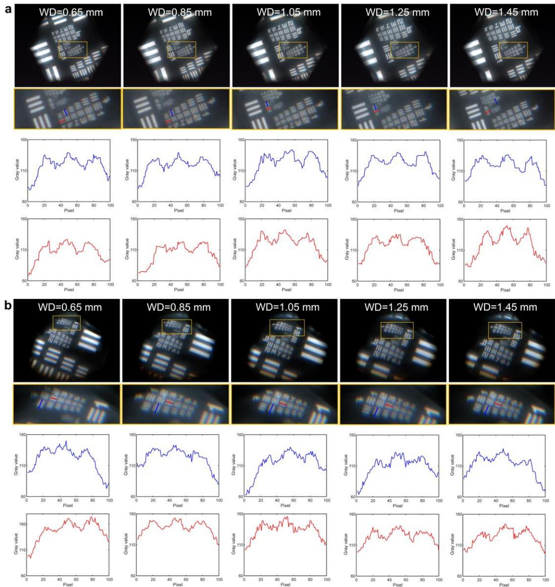
**Supplementary Figure S10 Resolution test with different working distances (WDs) at initial magnification of 18x. a** Resolution test results of the centre channel with different WDs at initial magnification of 18x. **b** Resolution test results of the edge channel with different WDs at initial magnification of 18x.
