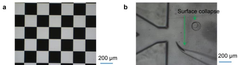
**Supplementary Figure S14 FOV of an ordinary microscope.** **a** Checkerboard image captured by the commercial microscope with 10× objective lens. **b** Microfluidic chip image captured by the commercial microscope.
