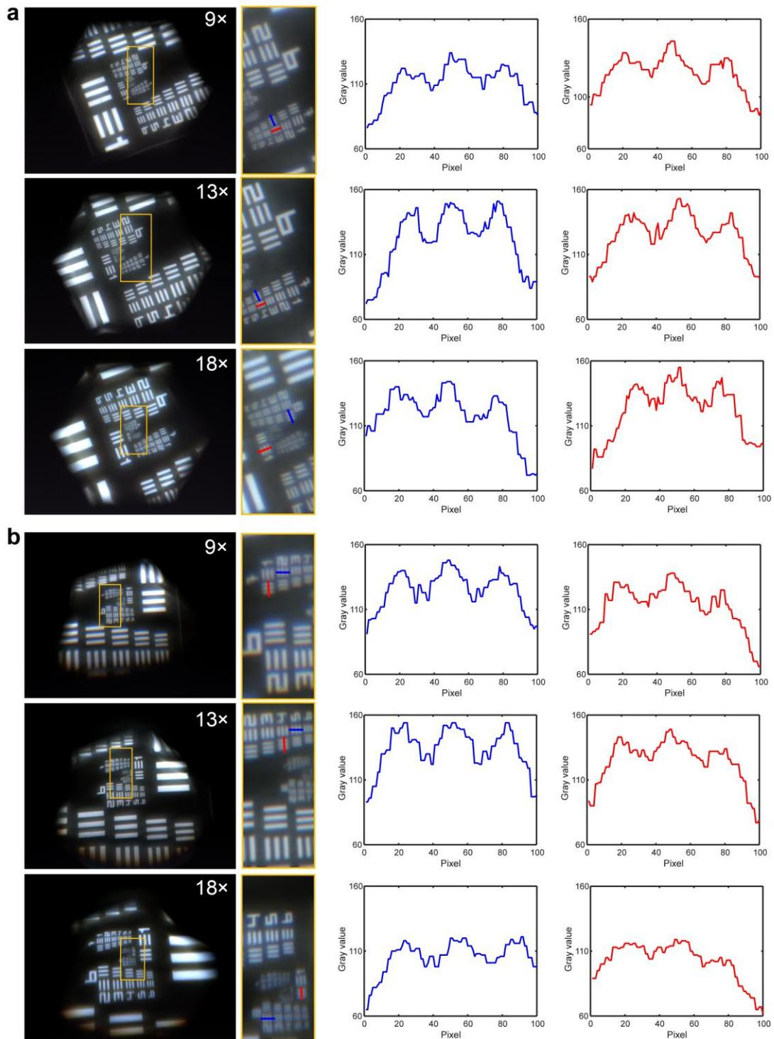
**Supplementary Figure S6 Resolution test at different magnifications. a** Resolution test results of the centre channel at magnifications of 9 $\times$ , 13 $\times$ , and 18 $\times$ . **b** Resolution test results of the edge channel at magnifications of 9 $\times$ , 13 $\times$ , and 18 $\times$ .
