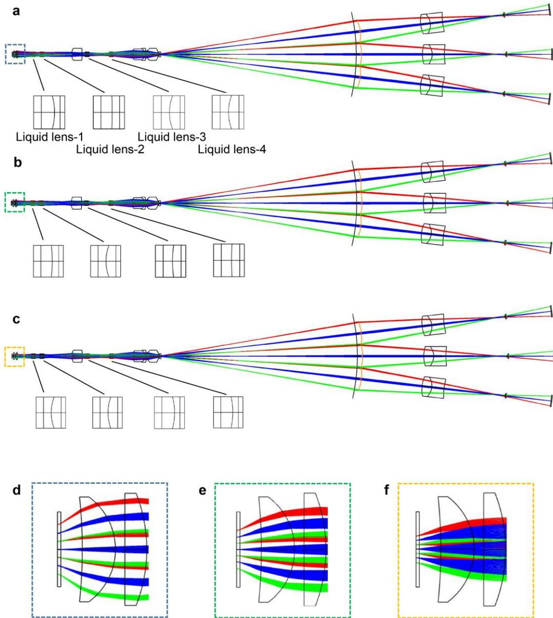
**Supplementary Figure S1 Optical path simulation of the proposed microscope. a–c** Simulated optical path of the microscope at magnifications of 9×, 13×, and 18×. **d–f** Local enlarged images of the simulated optical path at magnifications of 9×, 13×, and 18×.
