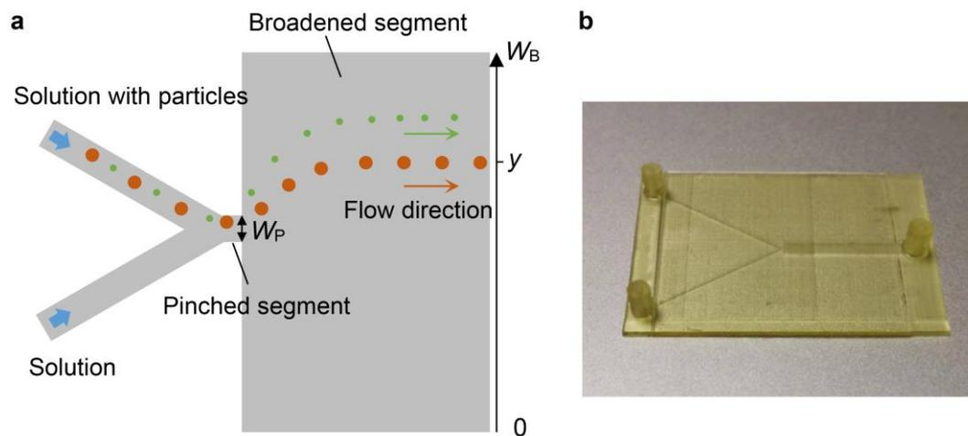
**Supplementary Figure S13 Principle and structure of the microfluidic chip for separation of particles. a** Principle of the microfluidic chip for separation of particles. **b** Real image of the microfluidic chip.
