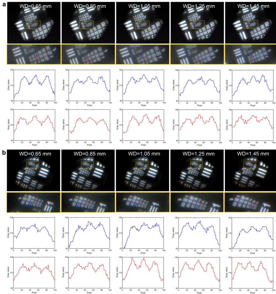
**Supplementary Figure S9 Resolution test with different working distances (WDs) at initial magnification of 13 $\times$ .** **a** Resolution test results of the centre channel with different WDs at initial magnification of 13 $\times$ . **b** Resolution test results of the edge channel with different WDs at initial magnification of 13 $\times$ .
