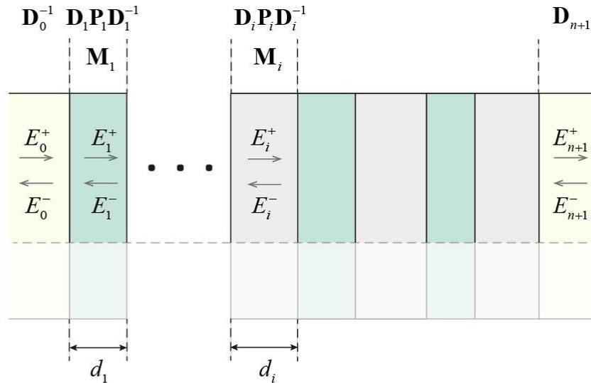
Fig. S1. The schematic view of multilayer thin films.
