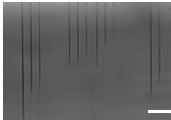
Fig. S4. The variation in nanohole length with respect to different pulse energies and number of pulses. (Scale bar: 50 \mu\text{m} )
