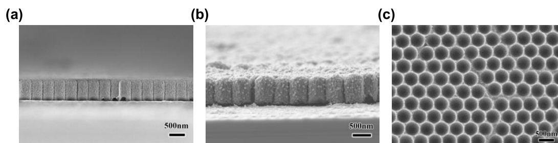
Figure S8. (a) Cross-sectional SEM image of a 500 nm-thick Cr film deposited using 400 nm polystyrene microspheres as the mask. (b) Cross-sectional SEM image of a 500 nm-thick Cr film deposited using 500 nm polystyrene microspheres as the mask. (c) SEM image of the back side of the sample after tape transfer.
