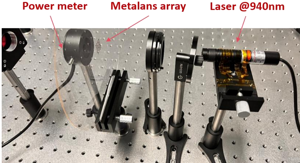
Fig S13 Diagram of the experimental setup for measuring the diffraction efficiency of a metalens
