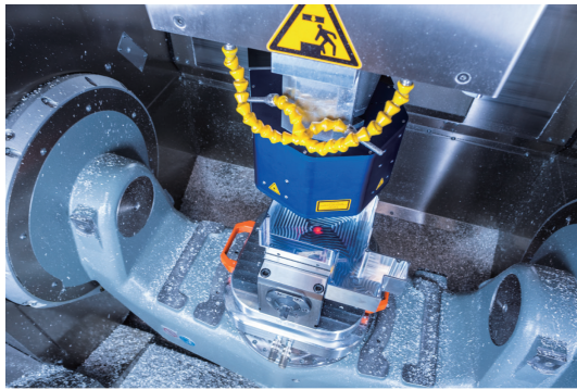
Fig. 7 Inspection of a typical milled surface by HoloPort in a Hermle C32U 5-axis milling machine at Fraunhofer IPM 19 .
